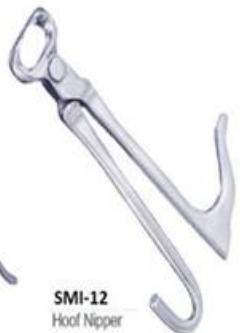
SMI-06 Hoof Nipper Size: 12" SPRING LOADED & Locking Nut Trimmer Premium Quality
